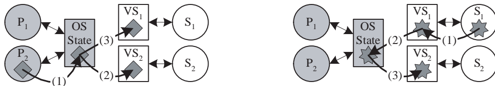
Figure 4.9. Foreground update and state propagation (left); idletime state commit at finish and propagation (right).
