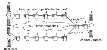
Fig. 1. Example topology with requesters on the left, original sources on the right, and potential caches along the path.
