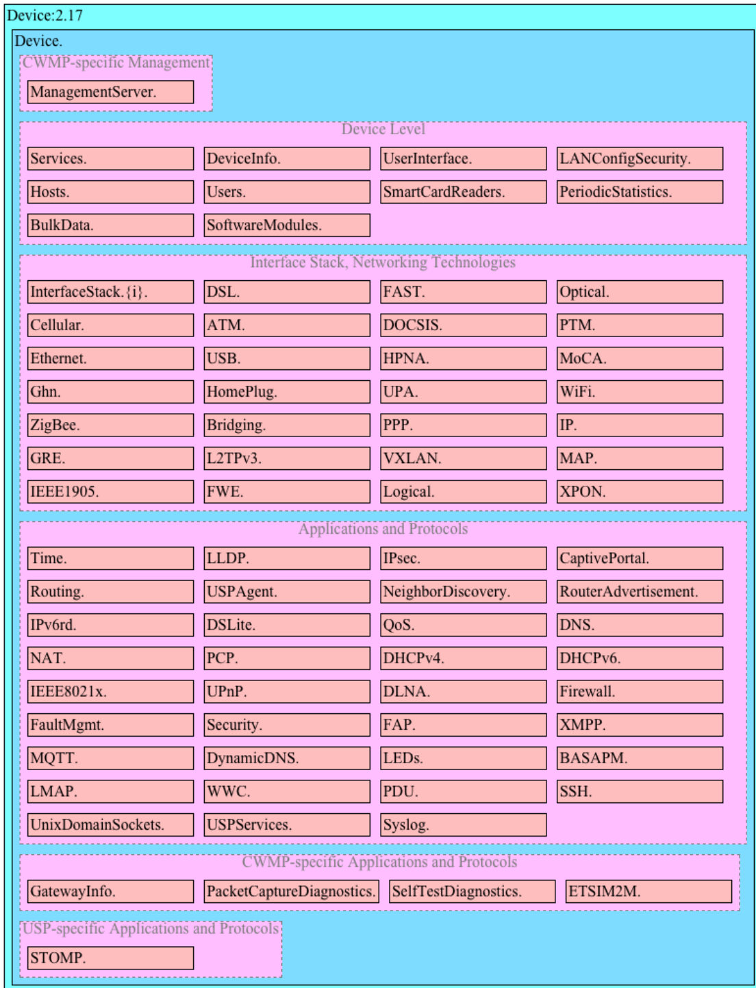
Figure 1: CWMP-specific Device:2 Data Model Structure – Overview
