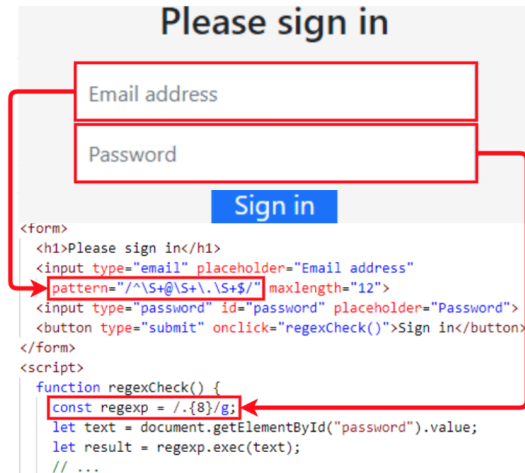
(a) Sanitization in HTML form. Regexes can be applied using an input field's pattern attribute, and via JavaScript event handlers.
