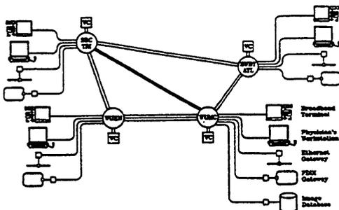
Application of fast packet switching to visual communication.
