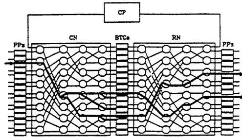
Routing Network (RN)—routes packets to proper output.
