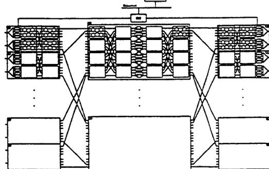
Packet Processor board includes 8 PPs with link interfaces and two eight port switch sections; four links multiplexed on single fiber.
