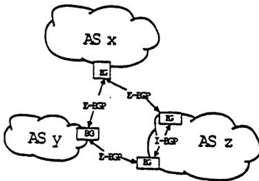
BGP testing simulating real Network
