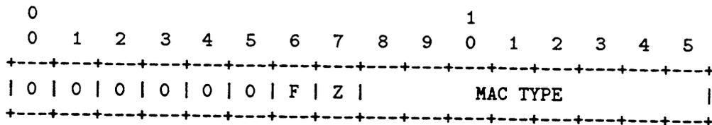
The F bit is used to indicate the presence of the MAC Frame Check Sequence, and the Z bit is used to indicate zero compression.
