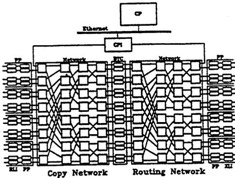
Copy and routing networks are implemented with single board having 32 PSE chips.
