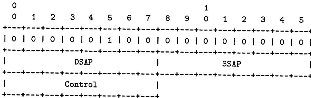
If the value of the Format Identifier is greater than 1024 decimal (0x0400) then the encoded Format Identifier is equivalent to the Digital-Intel-Xerox (DIX) Ethertype, as shown below.
