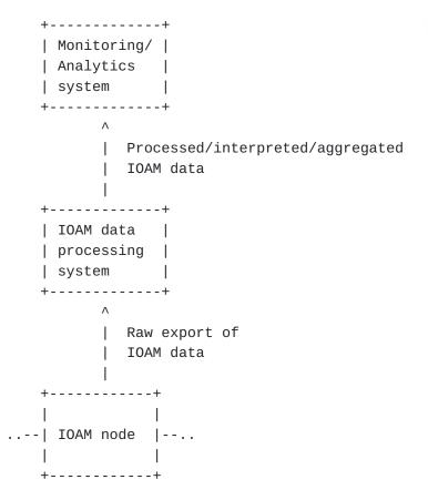
IOAM node: IOAM encapsulating, IOAM decapsulating or IOAM transit node.
