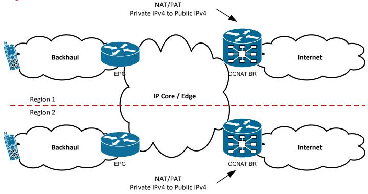
CGN performs NAT/PAT 44 - PAT substantially reduces Public and Private IPv4 address demand, but does not prevent IPv4 address depletion.
