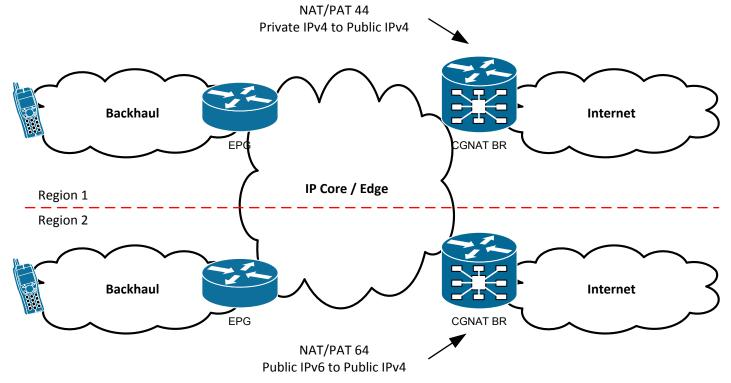
RFC1918 IPv4 Private Address space used for legacy UE assignment for each APN, and IPv6 GUA for IPv6-capable UEs CGN performs NAT/PAT 44 and NAT/PAT 64
