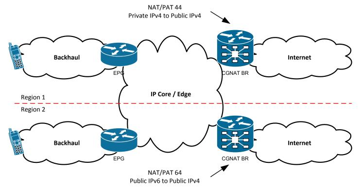
Backhaul is maintained as IPv4 transport Core is 6VPE Dual-Stack enabled
