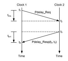
Fig. 5. Synchronization with peer delay mechanism
