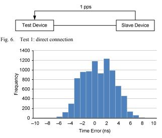
Fig. 7. Time error distribution for direct connection (Test 1)
