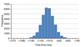
Fig. 12. Time error distribution for connection through a cascade of nontransparent switches (Test 3)
