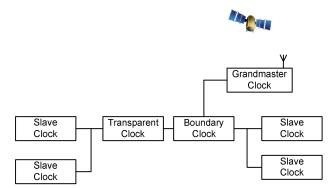
Fig. 2. Example PTP network topology
