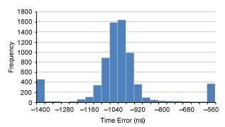
Fig. 14. Time error distribution with a cascade of three nontransparent switches and two GOOSE devices (Test 4)
