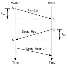
Fig. 4. Synchronization with delay request-response mechanism
