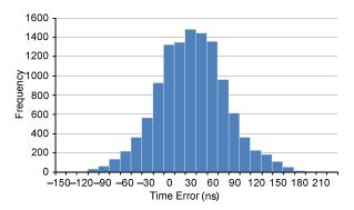
Fig. 17. Time error distribution for connection through a transparent switch (Test 5)
