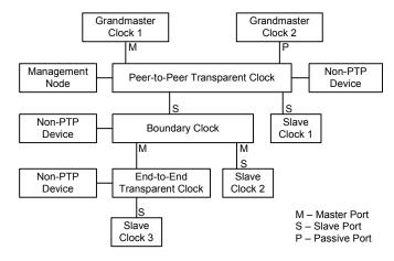
Fig. 3. Example PTP clock hierarchy
