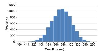
Fig. 10. Time error distributions for connection through a nontransparent switch with swapped connections (Test 2)
