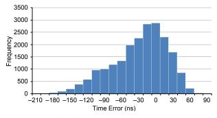
Fig. 18. Time error distribution for connection through a transparent switch with swapped connections (Test 5)
