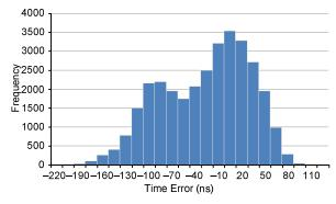
Fig. 20. Time error distribution with a transparent switch and two GOOSE devices (Test 6)
