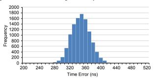
Fig. 9. Time error distributions for connection through a nontransparent switch (Test 2)
