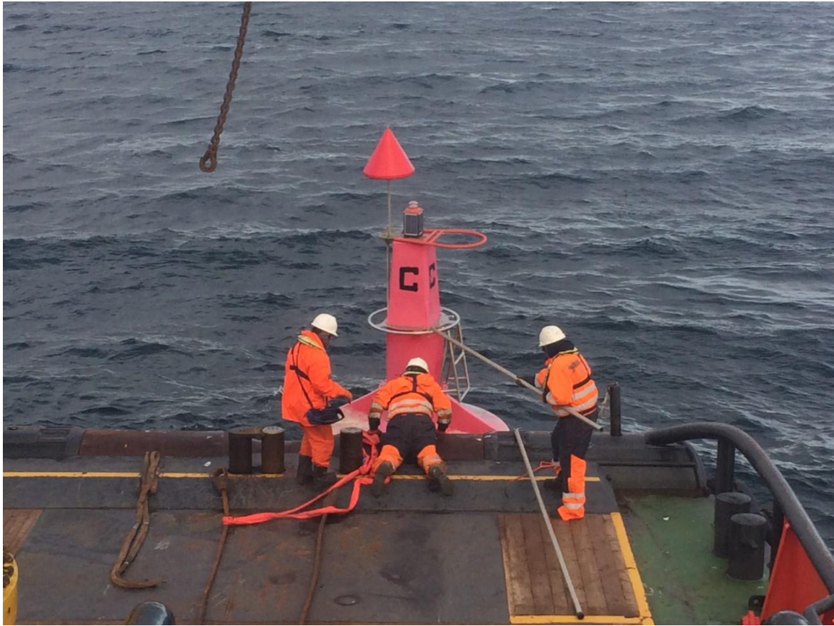
Picture 6 – Channel Marker Buoy undergoing maintenance at stern of tug.
