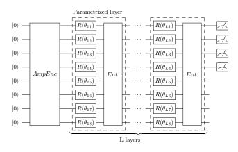
Fig. 9. Amplitude encoding circuit, where the encoding routine is depicted as a black-box unitary, followed by *L* parametrized *StronglyEntanglingLayers* and a final measurement of the first four qubits.
