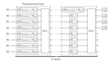
Fig. 8. Re-upload Encoding circuit used for the experiments in the main text. L StronglyEntanglingLayers are used encode the input and optimize over variational parameters, followed by measurements of the first four qubits.
