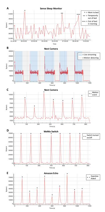
Figure 2: Network traffic send/receive rates of selected IP streams from 4 commercially-available IoT devices during controlled experiments. Clearly visible increases in send/receive rates directly correspond with user interactions.
