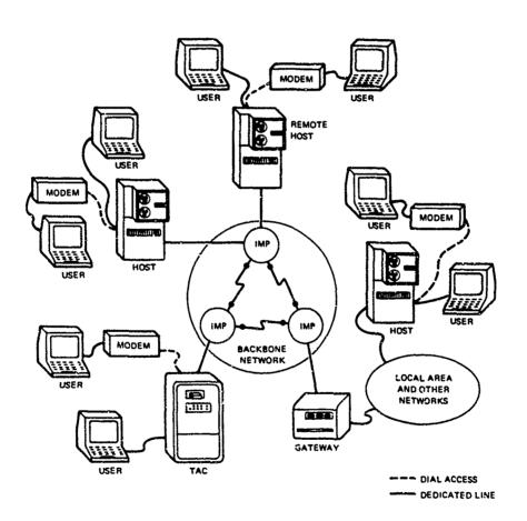
Figure 2-1: Hardware and Configuration of the DDN
