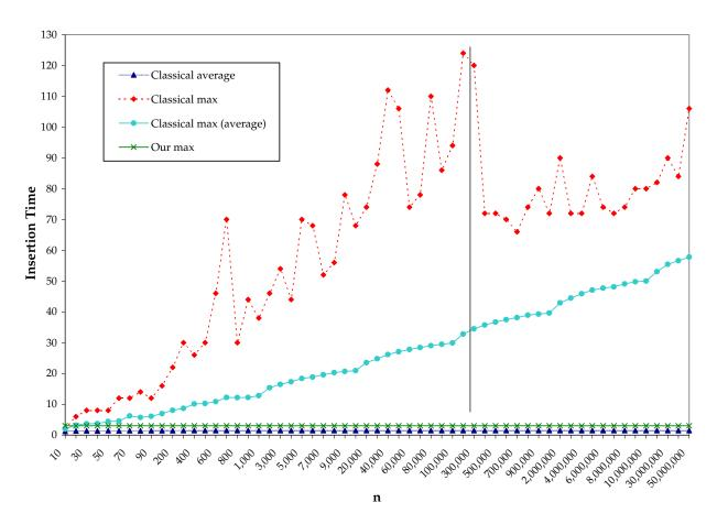
**Figure 5:** The insertion time of classical cuckoo hashing vs. our dictionary for  $\epsilon = 0.2$ .
