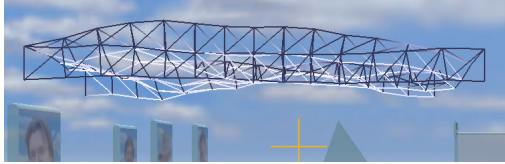
The wind starts the bridge oscillating
