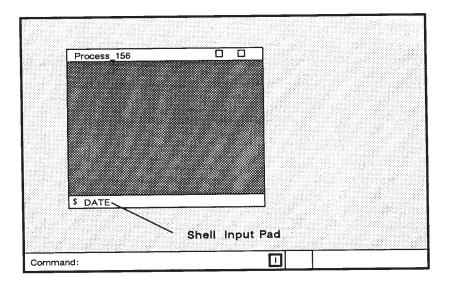
Figure 6-1. The Shell Process
