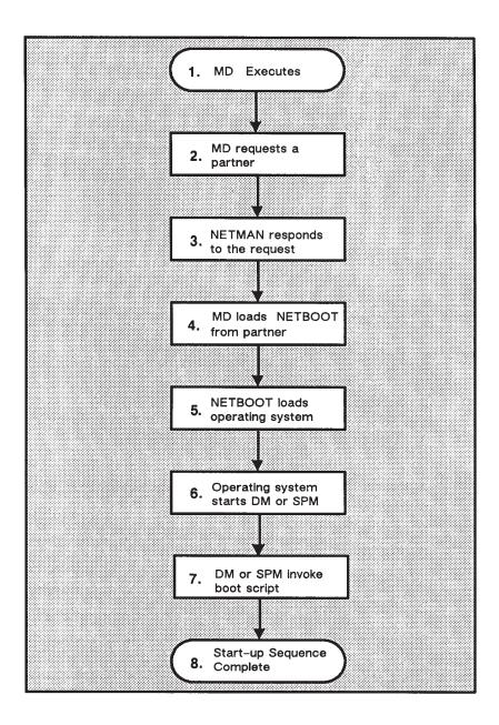
Figure 2-3. The Start-Up Sequence for a Diskless Node
