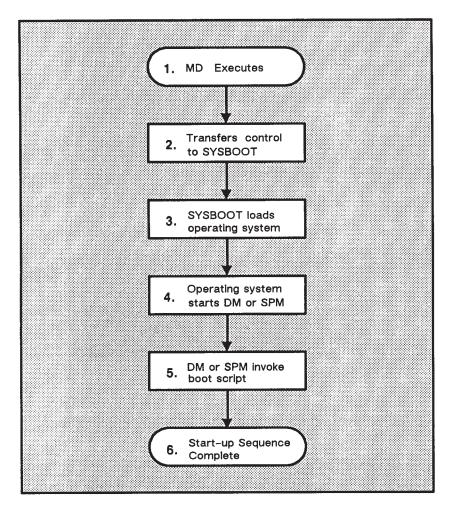
Figure 2-1. The Start-Up Sequence for Disked Nodes
