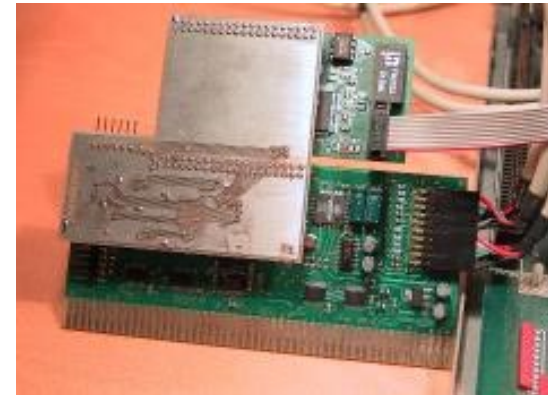
The prototype ROMulus module (on top) mounted on a Highway with a Norway Ethernet card on it's pass-through connector.
