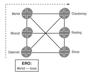
The opposite of a loose hop in an ERO is a *strict hop*. When you use a strict hop, you are informing the network of the exact path you wish the LSP to take. Each router examines the defined ERO and forwards the Path message to the next router listed. The next-hop router must be directly attached to the local router for this process to succeed.
