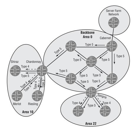
While the Type 5 LSA provides the network information necessary to reach the external networks, the OSPF routers may not automatically begin using that data. The address of the ASBR, Cabernet in our case, must be known in the link-state database via a router LSA. Chardonnay, Sangria, and the other backbone routers meet this criterion, because they share an area 0 database with Cabernet. It is the routers in area 10 and 22 that are currently not able to utilize the AS external LSA.
