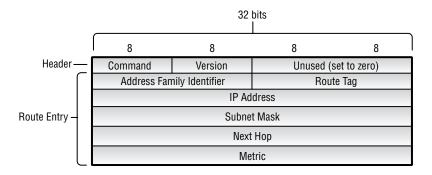
The RIPv2 header format is unchanged from RIPv1, except that the version number is now set to 2.
