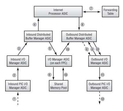
Let's use Figure 1.4 as a reference for the detailed steps of the unicast packet flow:
