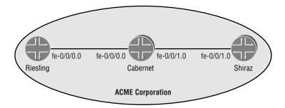
The following configuration for Cabernet allows it to receive RIP routes from both Riesling and Shiraz:
