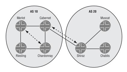
The Cabernet and Shiraz routers are joined by a direct physical connection. This connectivity implies that IP reachability is easily achieved between the two peers and that TCP can establish its session. On the other hand, the Merlot and Chardonnay routers are connected only via an intermediate router. In this situation, IP reachability between the peers must be supplied by some other means. Often this is handled by the IGP within the AS, but a static route is also a feasible solution.
