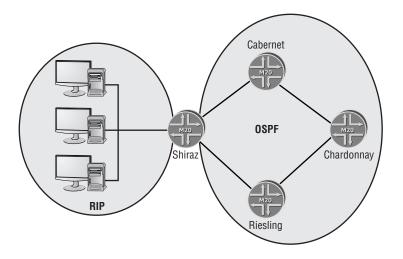
*Route redistribution* is a much more dynamic and scalable solution because it will allow the networks to expand without significant reconfiguration. To reach this goal, we place a routing policy on Shiraz to modify the protocol's default behavior. The policy allows the RIP process to advertise the OSPF learned routes and vice versa.
