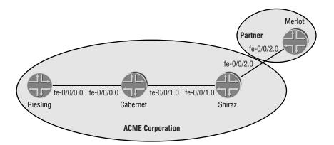
Merlot is able to communicate using the RIPv1 specification only, so Shiraz has added both the send and receive options within its neighbor statement for Merlot:
