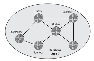
The Chablis router in area 0 is a backbone router with all interfaces within the area. This allows you to configure OSPF using two commands:
