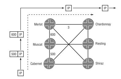
FIGURE 11.11 MPLS packet processing
