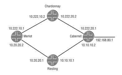
The currently assigned next hop for 192.168.80.1/32 is Riesling's interface of 10.20.20.1. Recall from the "JUNOS software Routing Table" section earlier in this chapter that a caret marker (>) designates the next hop installed in the forwarding table. The captures from Merlot clearly show this correlation. To install both 10.20.20.1 and 10.222.10.2 as next hops, we configure the following policy:
