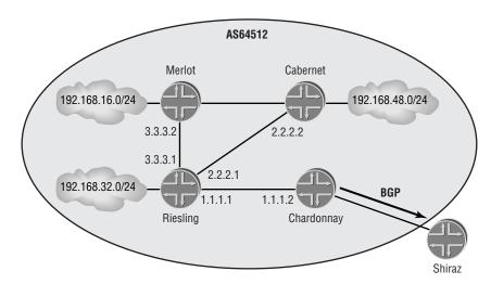
Riesling is communicating to the other routers in Autonomous System 64512 using the Intermediate System to Intermediate System (IS-IS) routing protocol. There are also static routes configured on Riesling that represent customers connected to that router. The current routing table looks like this:
