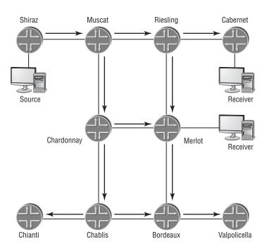
A quick look at Figure 9.9 shows that every router in the network doesn't need to receive the data stream. Only Merlot, Cabernet, and the routers along the path back to the source should be forwarding the traffic. Any router in a dense-mode network may prune itself from the forwarding path by sending a message to its upstream peer. This process occurs for all routers that do not need to receive the traffic.
