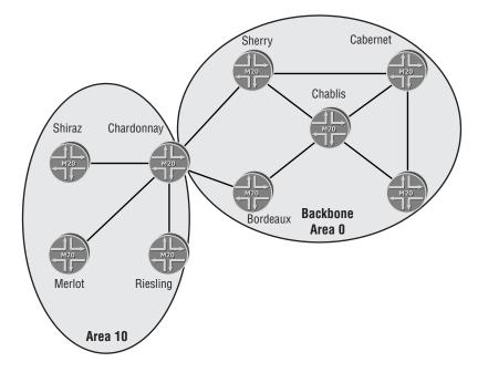
Our single-area network has grown and Chardonnay has become an ABR for area 10 with connections to the routers of Shiraz, Merlot, and Riesling. The configuration of Chardonnay for area 0 is already completed. We now add the interfaces within area 10:
