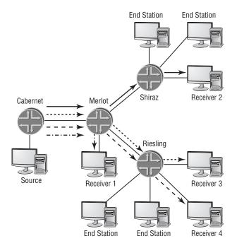
While the four receiving stations get their data traffic, we also burden the network needlessly. The Cabernet-Merlot and Merlot-Riesling physical links carry the same data multiple times, resulting in an overall loss of bandwidth in the network. Additionally, the routers themselves have to receive, process, and transmit additional packets. This could cause a resource drain within the router itself or congestion in the network as the outgoing interfaces fill up with the unneeded packets.
