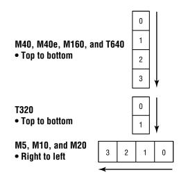
The vast majority of FPCs for a Juniper Networks platform contain four PIC slots (numbered 0 through 3). Some physical PICs are *quad-wide* and combine the PIC with an FPC in a single FPC slot. In this situation, the PIC slot number is always set to 0.
