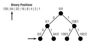
This second level of the tree has four possible binary values for the first octet: 00000000, 010000000, 10000000, and 11000000. These decimal values of 0, 64, 128, and 192 are represented by the IP addresses of 0 /2, 64 /2, 128 /2, and 192 /2 on the radix tree. This step-by-step
