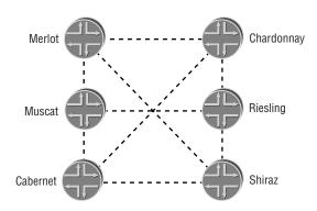
Each VC connection in the network appears as a point-to-point interface from the perspective of the router. In reality, however, the physical ATM connectivity may be quite different. Figure 11.4 shows this second set of connections.
