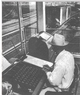
Teletype printer records individual freight car data in yard control tower.
