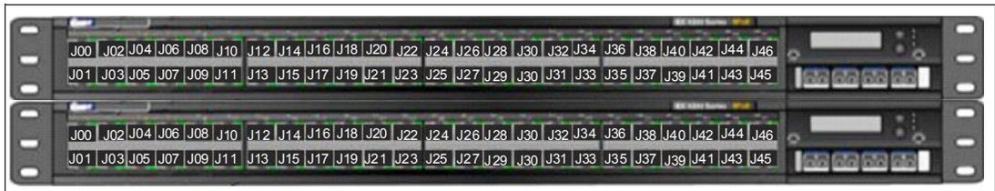
Figure 7-7 Two 1000BASE-T TOR switches
