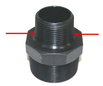
To accurately identify any BSPP or BSPT fitting, measure from one side of the thread to the other and refer to the chart above. EG: If the fitting measured 33.249mm across, it is a 1" BSP fitting and you would refer to it as a 1" BSP fitting. A 2" fitting would measure 59.614mm across the threads and therefore it is called a 2" BSP fitting.
