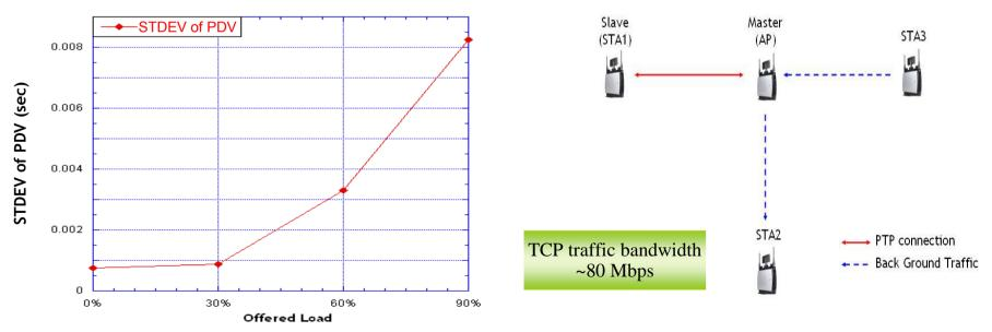
STDEV of Offset at Different Offered Load in Characterization Mode Back Ground Traffic Applied BSS Experiment Set Up
