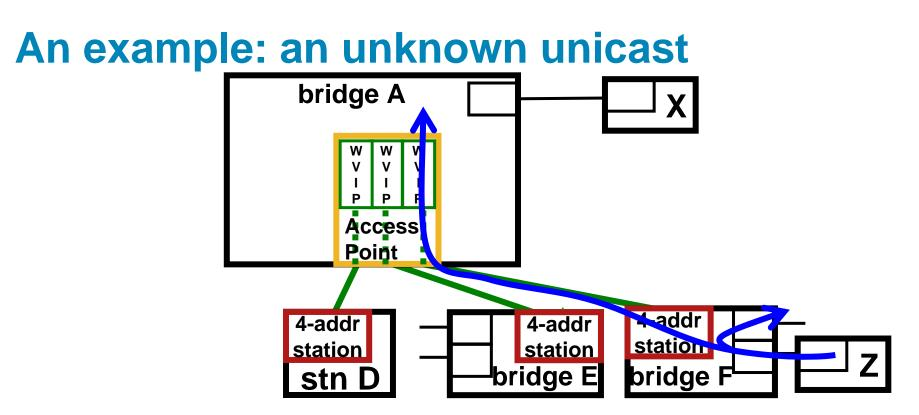
Suppose Bridge F relays an unknown unicast frame from Station Z to "W" via Bridge A (and to its other ports).
