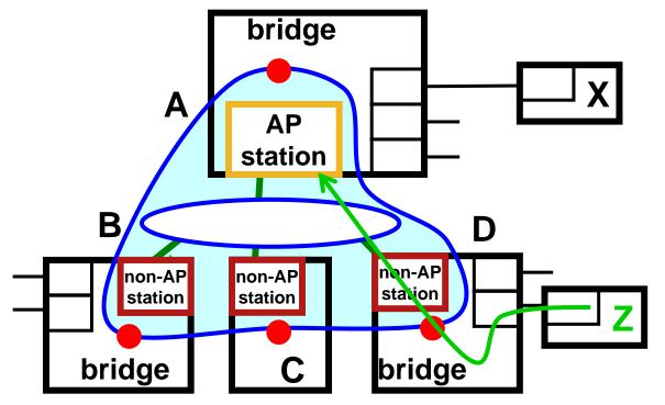
• The 802.11 four-address format can be used to signal ownership:
