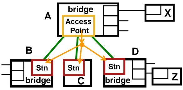
Let us, just for a moment, use the incorrect but commonly used terms for "station" and "access point", but separate the AP from the bridge in which it is embedded.
