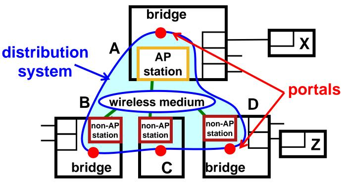
Among the requirements placed on a portal is the requirement that, if a multicast or broadcast is passed into the DS through a portal, it is passed to all of the other portals, but not back out the ingress portal.
