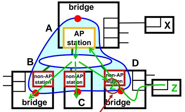
• We piggyback the data frame on the signal with the 4-address format:
