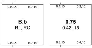
A template for and example of an STP Bridge. **B.b** is the Bridge Identifier (including the manageable priority component **B.**). **R.r** and **RC** are the Root Identifier, Root Path Cost, and the Designated Bridge Identifier, for the Root Port. **p.p**, **pc** are the Port Identifier (with manageable priority **p.**) and the Port Path Cost for a Bridge Port.
