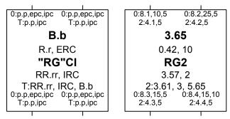
A template for and an example of an MSTP Bridge. **B.b** is the CIST Bridge Identifier. **R.r**, **ERC**, **RR.rr** are the CIST Root Identifier, External Root Path Cost, and Regional Root Identifier. **CI** identifies the Configuration Identifier for the Bridge. **RR.rr**, **IRC** the CIST Regional Root Identifier and the Internal Root Path Cost. **T:RR.rr**, **IRC**, **B.b**, is the Regional Root Identifier, Internal Root Path Cost IRC, and Bridge Identifier for the MSTI with MSTID **T**.
