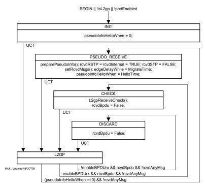
Figure 13-29—L2 Gateway Port Receive state machine
