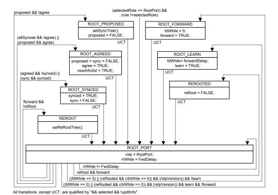
Figure 13-24—Port Role Transitions state machine—RootPort
