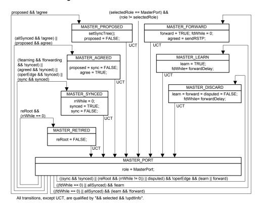
Figure 13-23—Port Role Transitions state machine—MasterPort
