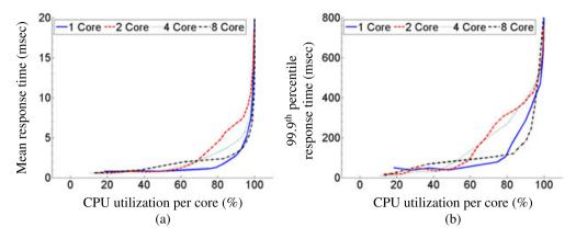
Figure 6. Web server response time versus CPU utilization for the Support workload: (a) mean and (b) 99.9th percentile.
