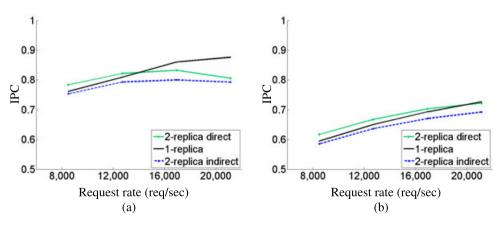
Figure 14. Instructions per cycle (IPC) versus request rate (req/s) with *1-replica*, *2-replica direct* and *2-replica indirect* configurations under (a) Support workload (RF = 0) and (b) Modified Support workload (RF = 0.6).
