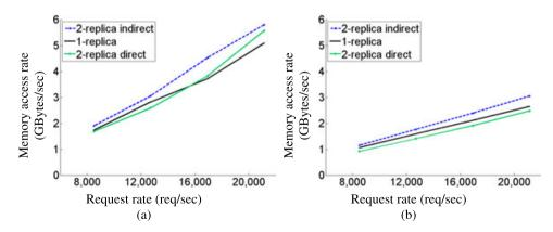
Figure 16. Memory access rate versus request rate (req/s) with *1-replica, 2-replica direct* and 2-*replica indirect* configurations under (a) Support workload (RF = 0) and (b) Modified Support workload (RF = 0.6).
