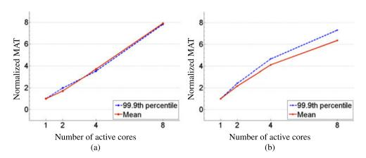
Figure 4. Normalized maximum achievable throughput (MAT) with one, two, four and eight active cores: (a) TCP/IP intensive workload and (b) Support workload.
