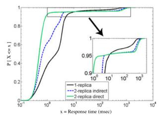
Figure 11. Cumulative distribution function (CDF) of response times in 80% CPU utilization with baseline and 2-replica configurations under the Support workload.
