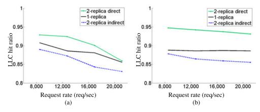
Figure 15. Last level cache (LLC) hit ratio versus request rate (req/s) with *1-replica*, *2-replica direct* and *2-replica indirect* configurations under (a) Support workload (RF = 0) and (b) Modified Support workload (RF = 0.6).
