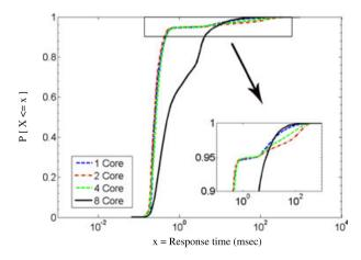
Figure 7. Cumulative distribution function (CDF) of response times at 80% CPU utilization for SPECweb Support workload.
