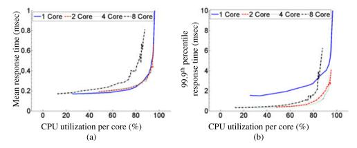
Figure 5. Web server response time versus CPU utilization for the TCP/IP intensive workload: (a) mean and (b) 99.9th percentile.
