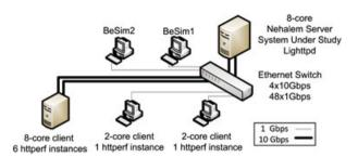
Figure 2. Testbed for Support workload.
