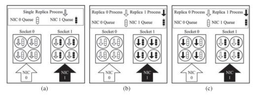
Figure 3. Network interface card (NIC) queue and Web server process mappings: (a) original, (b) direct mapping and (c) indirect mapping.
