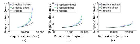
Figure 12. Web server response time versus request rate for Modified Support workload: (a) RF = 0.2, (b) RF = 0.4 and (c) RF = 0.6.
