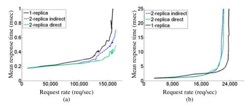
Figure 9. Web server response time versus request rate for eight cores with *1-replica* and *2-replica* configurations: (a) TCP/IP intensive workload and (b) Support workload.
