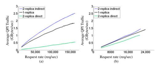
Figure 10. Average QPI traffic versus request rate for *1-replica* and *2-replica* configurations: (a) TCP/IP intensive workload and (b) SPECweb Support workload.
