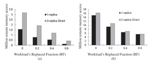
Figure 17. Total remote memory access per module for workloads with RF = 0, RF = 0.2, RF = 0.4 and RF = 0.6 with *1-replica*, *2-replica direct* and *2-replica indirect* configurations under (a) PHP-FCGI and (b) VMLinux.
