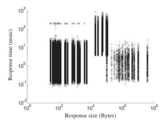
Figure 8. Response time versus response size for a test with eight active cores at 80% CPU utilization for the Support workload.
