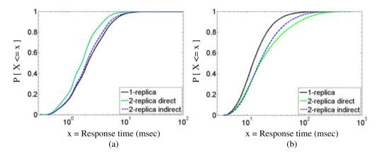
Figure 13. Cumulative distribution function (CDF) of response times in 80% CPU utilization for the synthetic mix with RF = 0.6 (a) static requests and (b) dynamic requests.
