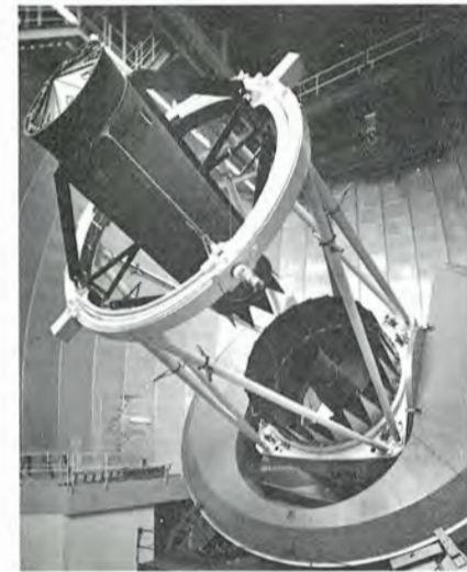
The Mayall telescope showing the 4-metre fused quartz mirror at centre of horseshoe (lower right) and prime-focus observing cage (upper left).
