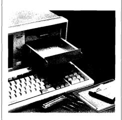
The HP R/332 Rack Mountable Controller offers HP VABs HP 9000 Series 300 performance and more: ruggedness, a compact transportable design, and rack mountability. For OEMs or other VABs, an extra added touch is the Al308A Custom Engineering Kit accessory, which allows customization of the front panel of the HP R/332 Controller. The kit can be easily configured either as a convenient storage drawer, or as a customized electronic I/O panel.
