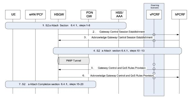
*Figure 25* Initial attachment over S2a
