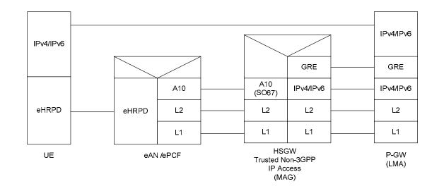
Figure 5 Protocol stack for non-multiplexed traffic on an Auxiliary Connection
