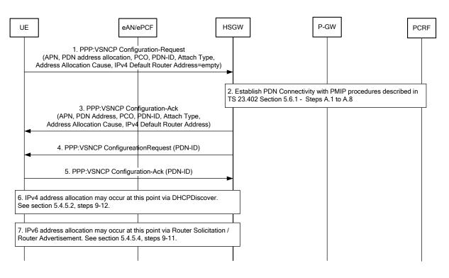
Figure 27 UE Requested Additional PDN Connectivity
