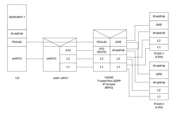
Figure 4 Protocol stack for traffic multiplexed on an SO72 Auxiliary Connection
