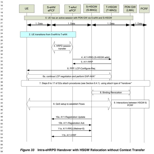
0. The UE has an active session up and running with the P-GW via the source eAN/ePCF (S-eAN/ePCF) and source HSGW (S-HSGW).
