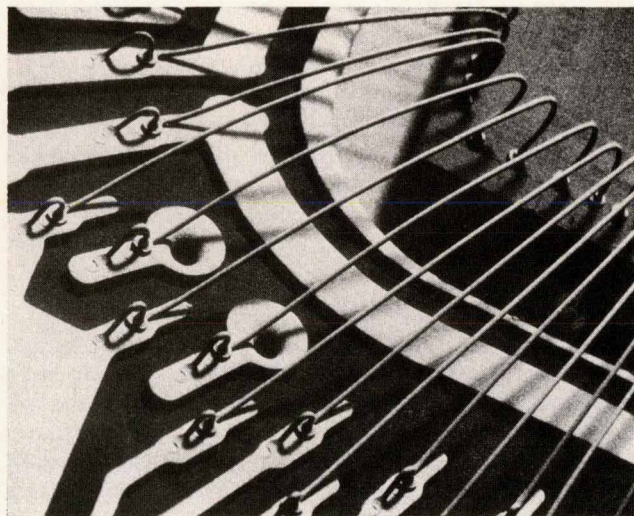
Fig. 2. Wire bonds from the IC to the finstrate use an extra ball bond over the tail bond as shown.
