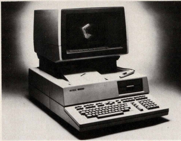
Fig. 3. The HP 9000 Computer uses HP's new VLSI and finstrate technologies to provide a desktop-size workstation low enough in price to let professional personnel have their own personal 32-bit mainframes.
