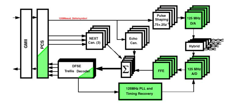
Blocks common between a Quad 100Base- TX and a 1000BASE-T transceiver. NEXT and Echo cancellers are the major blocks contributing to the added complexity over a Fully digital Quad-TX.
