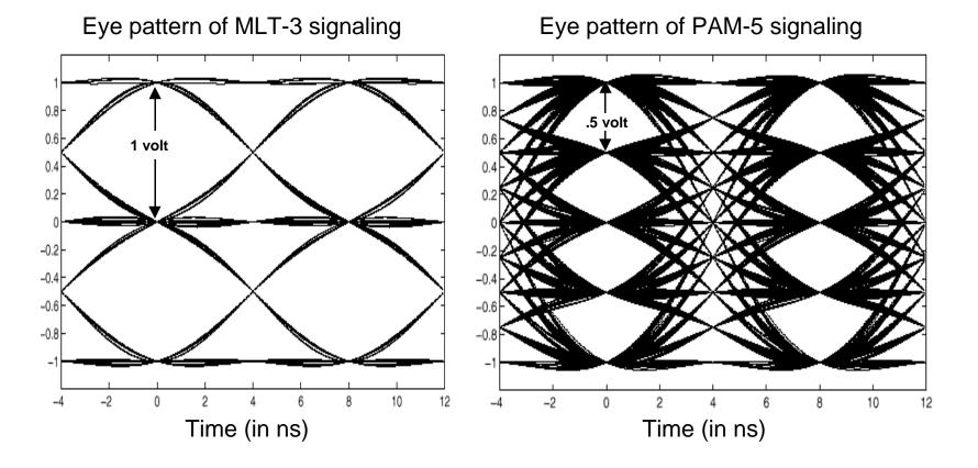
Recover the 6dB of SNR -- Add Forward Error Correction (FEC)
