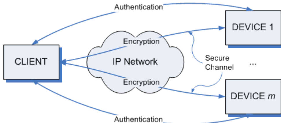
1018 1019 Figure 2: Communication mechanisms for authentication information and for encrypted messages 1020 The organization of CLIENT and DEVICE credentials, mechanism for provisioning them, and criteria for 1021 distinguishing valid and invalid credentials is out of scope of this profile.
